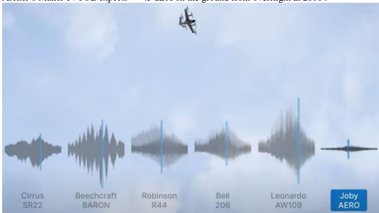
Fig. 1. Noise (dBA) traces as common fixed- or rotary-wing aircraft, or a Joby electric air taxi, overfly the listener under identical conditions. Graphic courtesy of Joby (see endnote reference).
